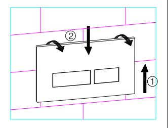
Disassembly: As per illustration ①, push the button plate upward and then pull it out as per illustration ②.
